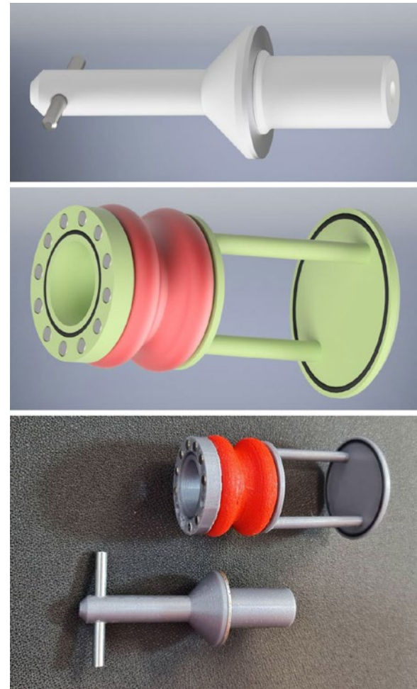
Figure 4. Three-part airlock for sampling (above: Handpiece/swab holder; middle: piston insert with sealing ring; bottom: printed components)
