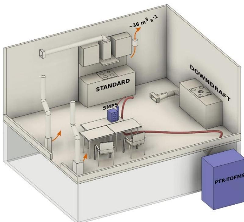
**Figure 3.** Testroom setup with advanced real-time measurements.
