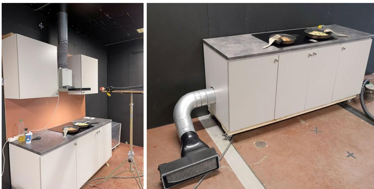
**Figure 2.** Ducted standard setup (left) and downdraft recirculating solution (right).
