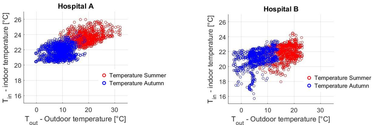
**Figure 4.** Comparison between indoor and outdoor temperature for hospital A (a) and hospital B (b) based on mean hourly data of all measured rooms.
