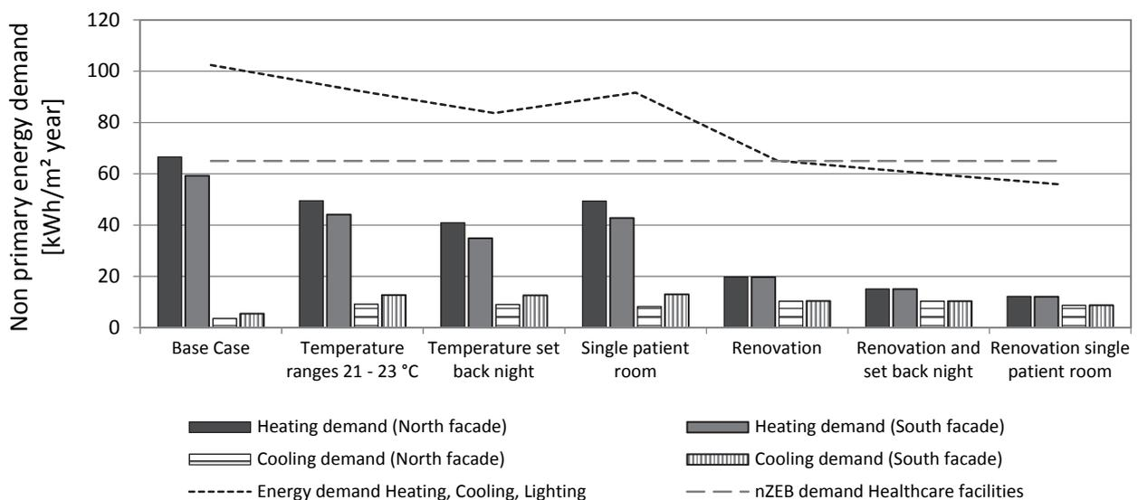
**Figure 5.** Heating and cooling demand per square meter for different scenarios with heating and cooling set-point of 23–25°C for the base case and 21–23°C for the other scenarios. For the scenarios with temperature set back, heating set point is 18°C during the night (9:00 p.m. – 6:00 a.m.).
