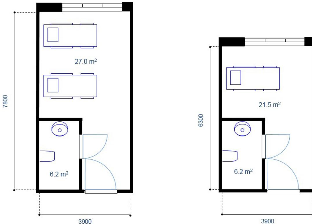
**Figure 3.** Floorplan of a two-bedded room and single bedded room used for the simulations.
