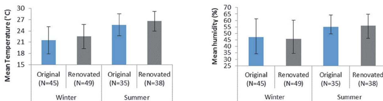
**Figure 1.** Average indoor temperature (left) and humidity (right) in the bedrooms of the investigated during the winter and summer season. Ends of the whiskers characterises the minimum and maximum values.
