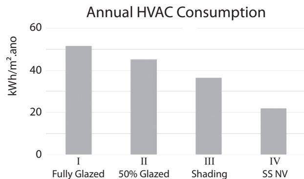
**Figure 5.** HVAC consumption for an averaged floor.
