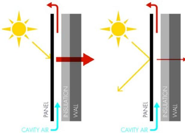
**Figure 5.** Conventional (left) and spectrally selective (right) facade coatings.
