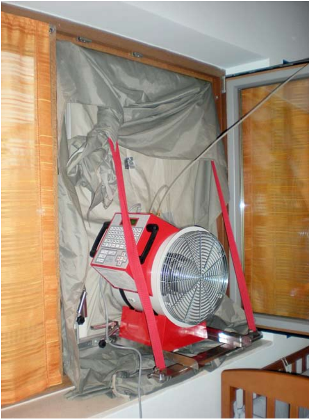
Figure 4. Blower Door test.
