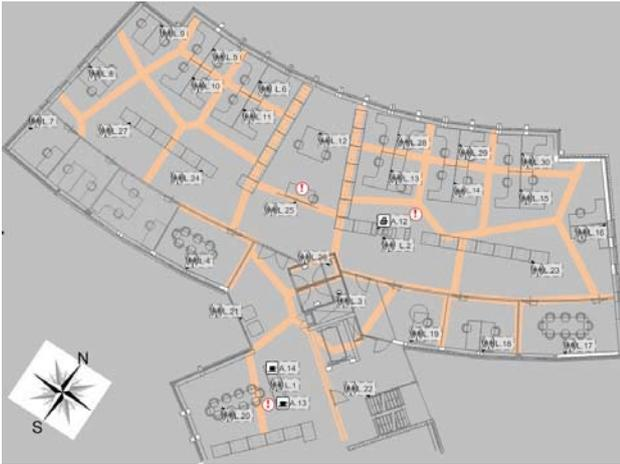
**Figure 6.** Positions of the static nodes creating a mesh of the zones for measuring the position of the building occupants on the floor. The transition region between the zones is marked by the broad orange line.
