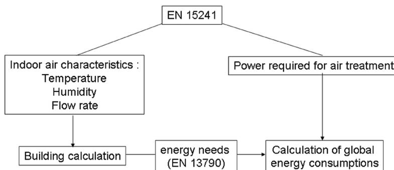
Figure 1. Basic principles of the use of EN15241 in relation to EN13790
