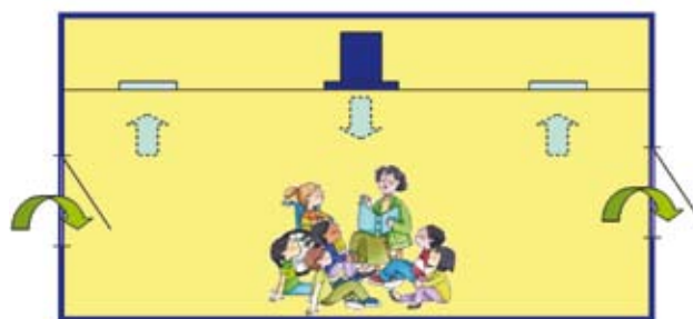
Figure 1. Hybrid ventilation system: concept of concurrent operation
