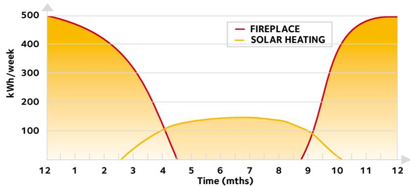
**Figure 4.** Solar heating and heating generated with a fireplace can complement one another. Regular heating of the fireplace is the natural alternative during the winter months, when the need for heating energy is highest. Solar heating is the most effective in early spring and in summer when the heating energy produced can be used for floor heating in wet rooms and for domestic hot water. Such combination will minimise the delivered electricity use.
