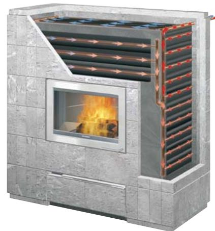
**Figure 5.** The Sonka accumulating soapstone fireplace equipped with heat exchangers.
