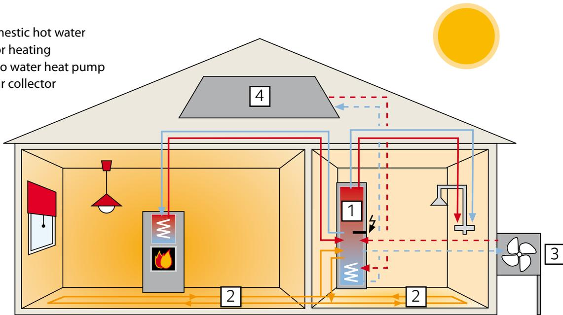
**Figure 2.** A fireplace with heat exchangers integrated into water-based heating systems.
