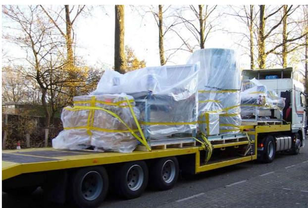
Figure 10. Plant room packed and ready for transportation.
