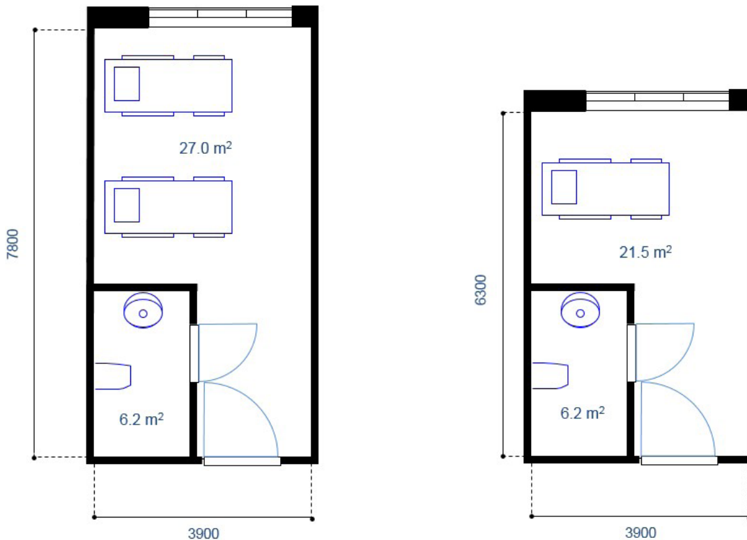
Figure 3. Floorplan of a two-bedded room and single bedded room used for the simulations.
