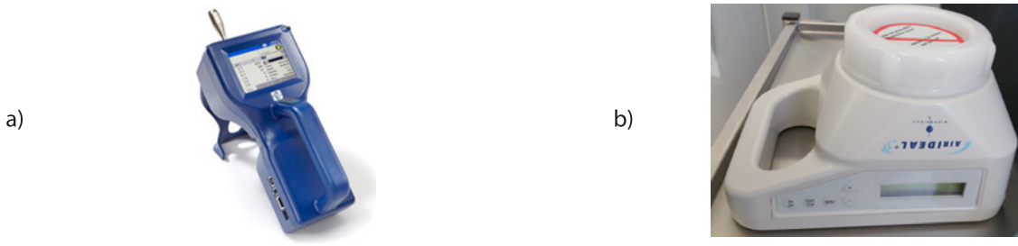
Figure 3. Measurement instruments, a) AEROTRAK™ Handheld Particle Counter Model 9306, b) CFU measurement device.
