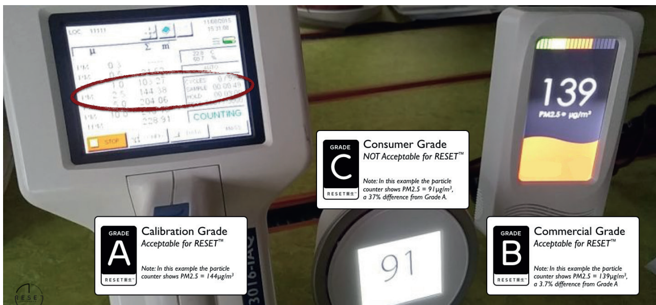
Figure 4. Varying accuracy of three monitors show the difference between monitor quality grades. General rule: if you can't calibrate it, don't buy it. Only Grade A and Grade B monitors are accepted for RESET™. Latest RESET™ standards are here: http://reset.build/resources/RESET_Accredited_Air_Monitor_Requirements
