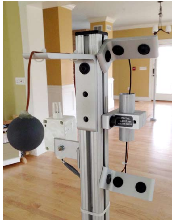
Figure 2. Test stand for measurement of thermal comfort parameters.
