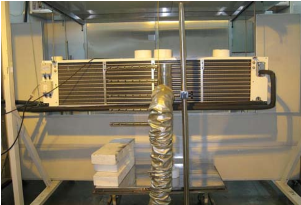
Figure 1. CO 2 evaporator testing.
