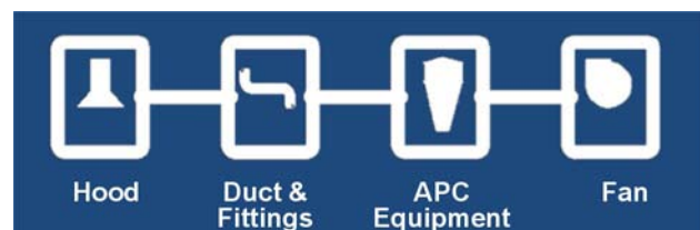
Figure 2. System design components.
