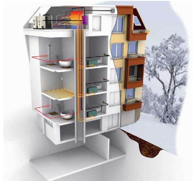
Figure 5. A centralized heat pump in an apartment building. [Courtesy of Robur]
