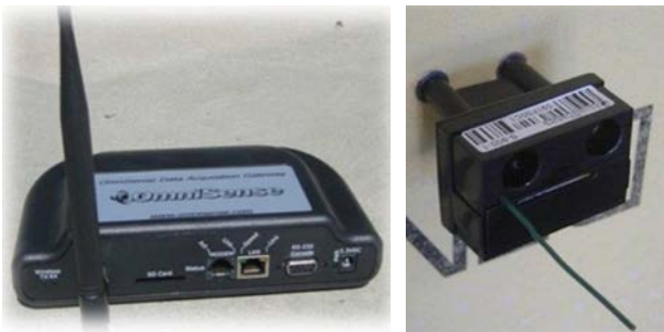
Figure 6. Omnisense, S-900-1, Wireless T, %RH, WME Sensor.
