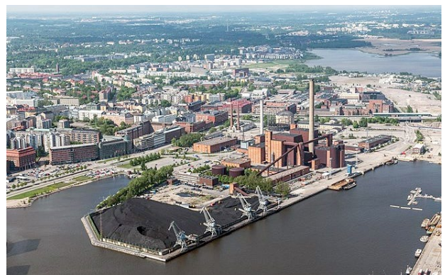
Buildings in Helsinki are mainly heated by coal fired district heating power plants. City will abandon the coal fired plants by 2029, and is looking new solutions with the open competition.
