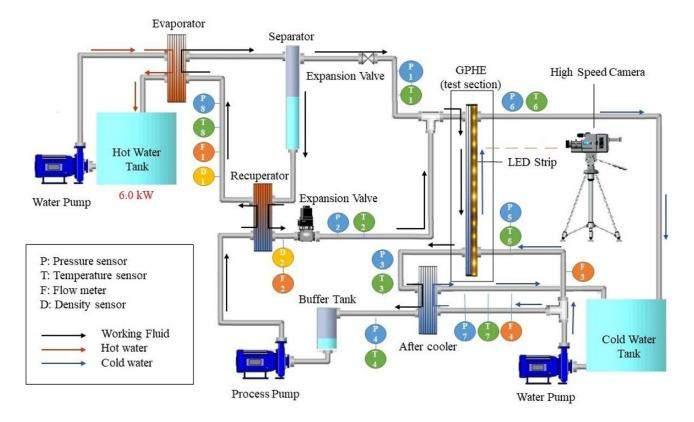
Figure 1. Experimental setup diagram of OTEC demo cycle.
