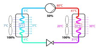
Figure 9. 50% load operating condition, if condenser fan modulates.
