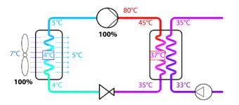
**Figure 4.** Example of part load operating conditions for the same air to water heat pump.
