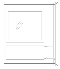
**Figure 2.** A properly dimensioned radiator has a large heat radiating surface. Radiator replacement is simplified when the connection pipes from the risers to the radiator valves are renewed if possible.
