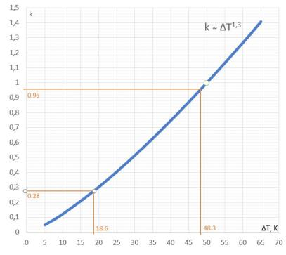
**Figure 3.** Dependence of radiator output ratio k on excess temperature  $\Delta T$ . For example, the radiator output at an excess temperature  $\Delta T$ 18.6K ( $T_{flow}/T_{rtn}/T_{in} = 45/35/21^{\circ}$ C) can be calculated using a diagram when the radiator output is known at another excess temperature, for example  $\Delta T$ 48.3K (80/60/21°C) the output is 1000 W. New output is obtained: 1000 W  $\cdot$  0.28/0.95 = 295 W.
