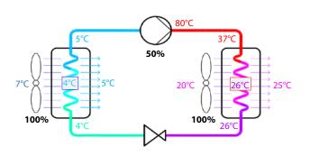
**Figure 8.** 50% load operating condition, coherent with path B assumptions and **Figure 5** full load conditions.
