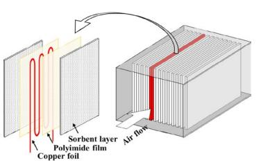
**Figure 1.** Illustration of the surface temperature adjustable laminated plate structure (left) and the air purifier module comprising multiple parallel plates (right). (Chen et al., 2019)
