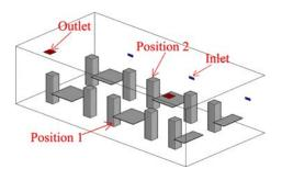
b) Stratum ventilation (SV) Three inlets: 0.30 m  $\times$  0.10 m (L  $\times$  W), 1.3 m above floor
