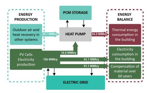
Figure 2. The overall energy balance of the ZEB Laboratory. [5]
