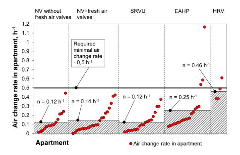
**Figure 1.** Air change rates measured in apartments renovated 2010-2014. Measurements made after operation for about one year after handing over (Mikola et al. 2022).
