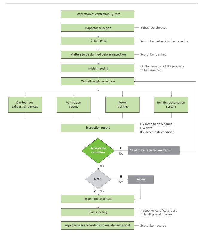
Figure 1. Stages of the walk-through inspection.
