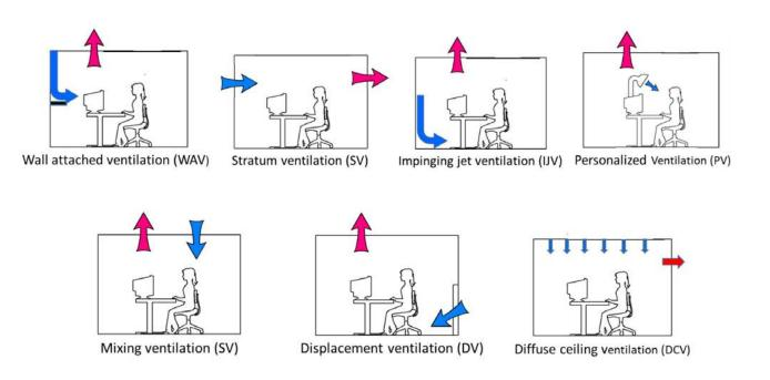
Figure 3. The simulated air distribution methods (blue arrows: supply; red arrows: exhaust).
