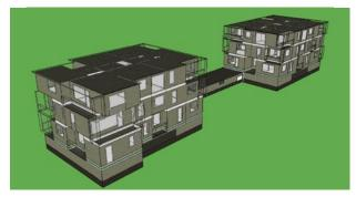
Uwall=0.14; Uroof=0.12; Ufloor=0.14; Uwindow=0.9; q50=1.5 m<sup>3</sup>/hm<sup>2</sup>. Heat recovery ventilation, 80% temp.ratio, electric reheating coil. No cooling (passive measures to control summer thermal comfort). Heat source options: DH (district heating), Gas (gas boiler), GSHP (ground source heat pump) and AWHP (air to water heat pump).
