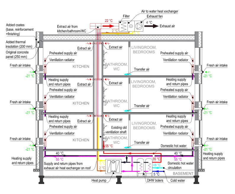
Figure 6. Ventilation radiators with exhaust heat pump heat recovery.
