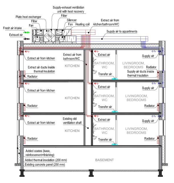
Figure 4. Working principle of centralized HRV renovation solution.
