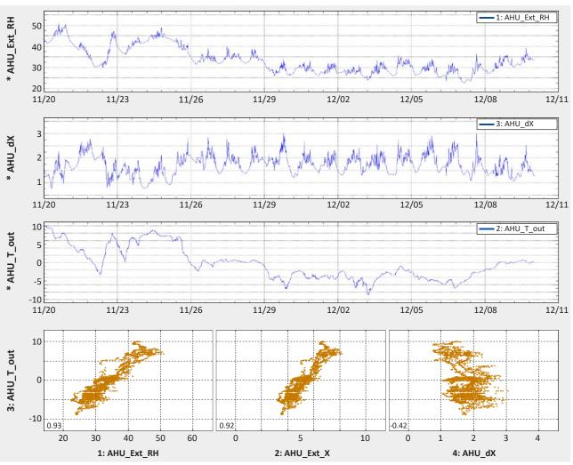
Figure 2. Extract air relative humidity, RH, extract moisture content, X, moisture generation, dX and outdoor temperature for an AHU investigated 20 November – 10 December 2021.
