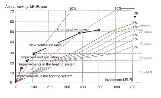
Figure 1. A package of energy saving measures in the IRR graph. The package did lead to 50% annual saving of energy.
