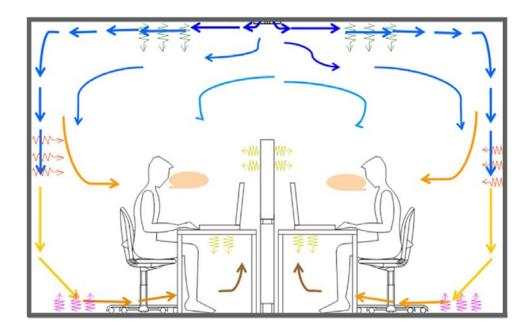
**Figure 1.** Mixing ventilation. Pollution generated by building materials and office equipment is mixed with the supplied clean air, transported to occupied zone and inhaled by occupants.
