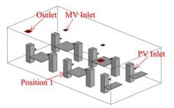
d) Personalized ventilation (PV) combined with MV MV inlet:  $0.25 \text{ m} \times 0.25 \text{ m} (L \times W)$ ,
