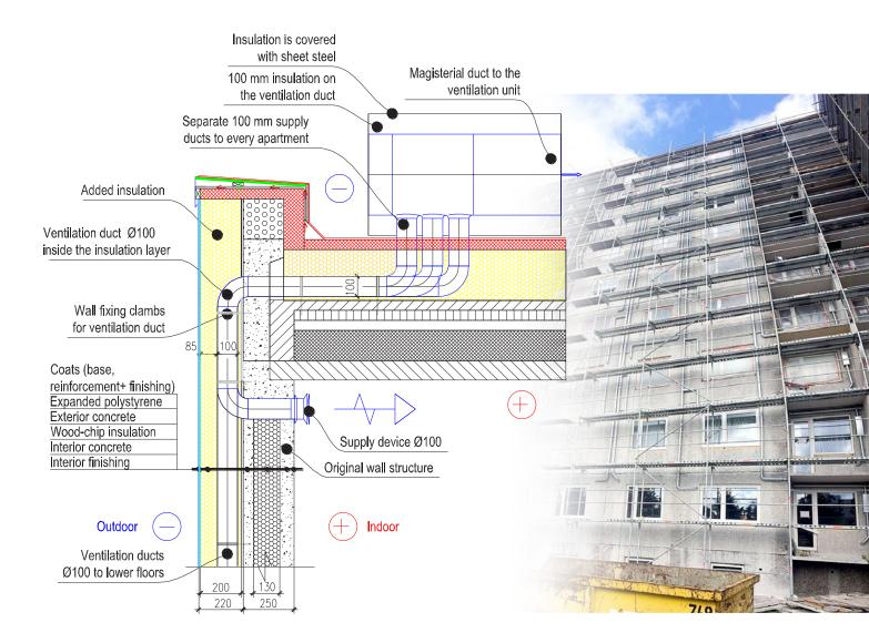
Figure 5. Ventilation ductwork installation on the wall.
