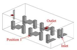
c) Impinging jet ventilation (IJV) Semi-circular inlet: radius 0.15 m, 0.95 m above floor
