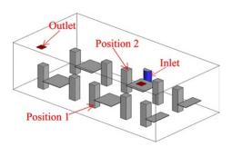
**f)** Displacement ventilation (DV) Semi-circular inlet - radius 0.25 m, height 0.97 m
