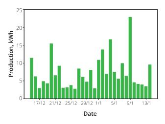
**Figure 4.** Daily PV production of the whole PV system during the investigated period.
