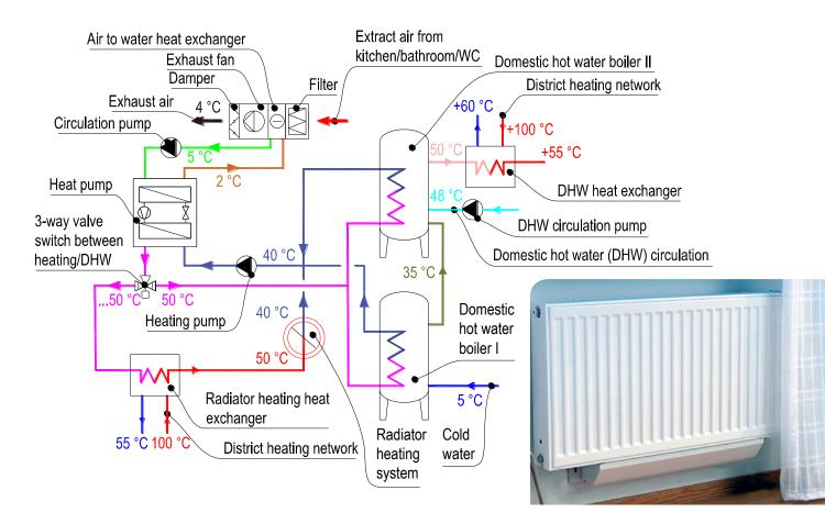
Figure 7. Exhaust air heat pump connection scheme and ventilation radiator.
