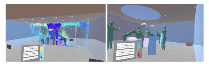
Figure 1. Visualization of airflow field (left) and airborne particle distribution (right) within the enclosed environment.
