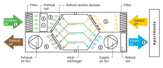
Figure 1. Principle sketch of residential AHU with counter flow heat exchanger:
