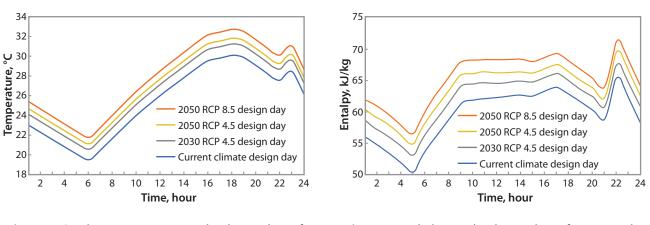
Figure 3. Outdoor temperature on the design days of Vantaa with 1% risk level.
