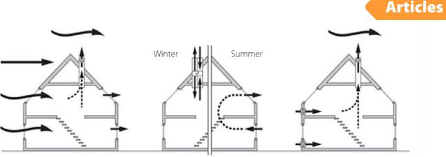
Fan supported natural ventilation Natural and mechanical ventilation Natural supported mechanical ventilation
