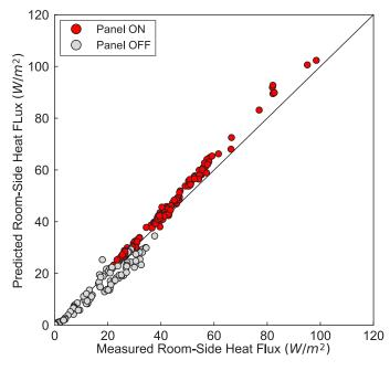
Egure f. Comparison of measured and predicted heat flux.
