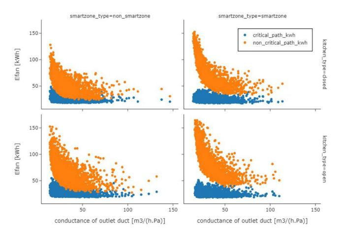
**Figure 3.** Average fan consumption (kWh) as a function of the outlet duct conductance (m<sup>3</sup>/(h.Pa)) for four cases (closed/open kitchen and Smartzone/non-Smartzone). Ventilation system based on critical or non-critical path control.
