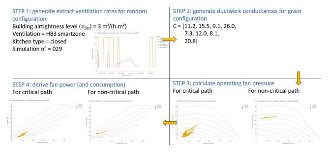
**Figure 1.** Flow of a single simulation. This example is simulation n° 29 out of 100 for the house configuration consisting of a closed kitchen, a building airtightness level of 3 m<sup>3</sup>/(h.m<sup>2</sup>), and a HB3 Smartzone ventilation system.
