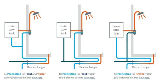
Figure 4. Hydraulic connection possibilities of a WWHR device.
