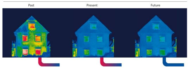
Figure 2. Illustration of the thermal development in building technology as an infrared thermography.
