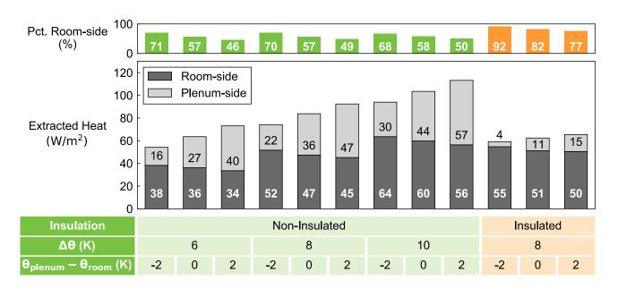
Figure 2. Heat extraction from the room and plenum by the non-insulated and the insulated panels.
