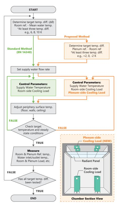
Figure 1. Standard and proposed cooling capacity measurement flow.
