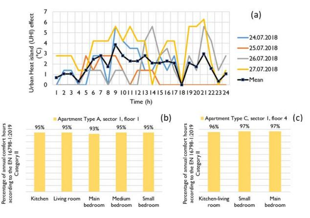
**Figure 2.** Measured urban heat island effect for different summer days (a) and percentage of annual comfort hours according to the EN 16798-1:2019 Category II for different apartment types: A (b) and C (c).
