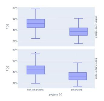
**Figure 4.** Boxplots of reduction factors obtained for four cases (closed/open kitchen and Smartzone/ non-Smartzone). Reduction factor = average fan consumption critical path control divided by average fan consumption non-critical path control.
