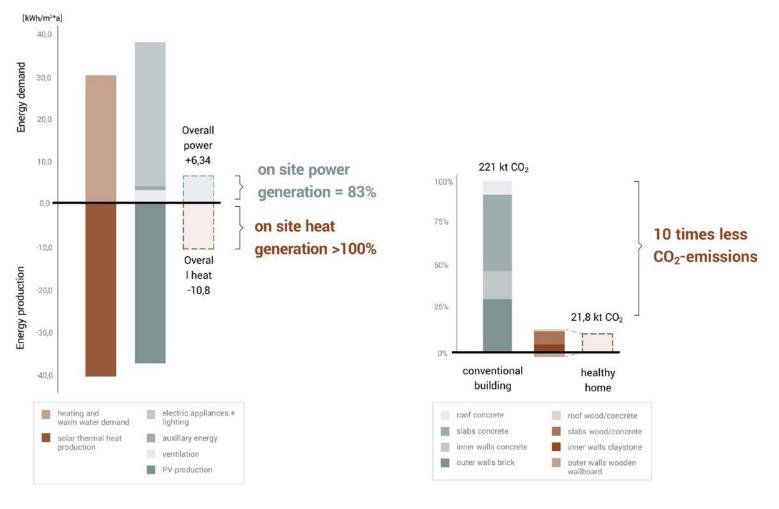
**Figure 5.** Comparison of energy demand and production (left) – the building is independent from supplied heat energy due to the seasonal warm water storage; comparison of CO<sub>2</sub>-equivalents of the load bearing structure of a conventional construction and the Horizontal Living project (right).
