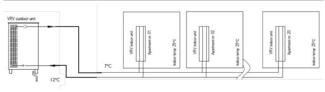
Figure 5. VRV cooling system scheme used for each apartment.
