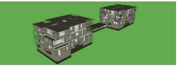
Uwall=0.14; Uroof=0.12; Ufloor=0.14; Uwindow=0.9; q50=1.5 m<sup>3</sup>/hm<sup>2</sup>. Heat recovery ventilation, 80% temp.ratio, electric reheating coil. No cooling (passive measures to control summer thermal comfort). Heat source options: DH (district heating), Gas (gas boiler), GSHP (ground source heat pump) and AWHP (air to water heat pump).
