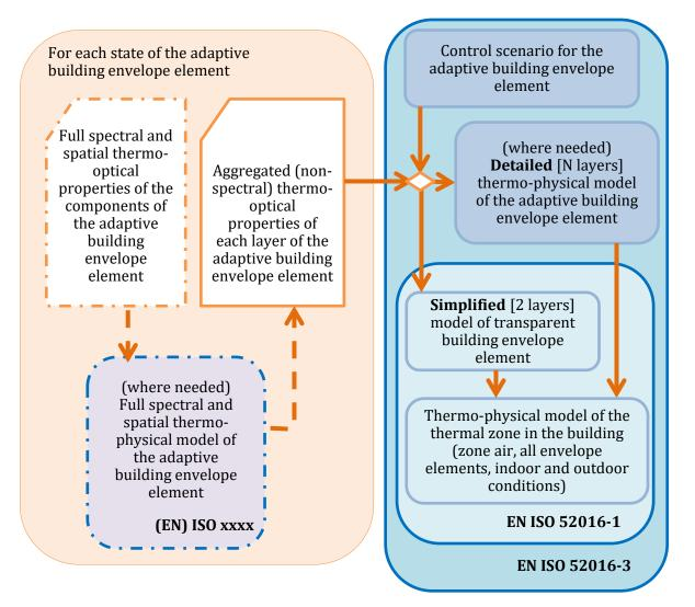
**Figure 2.** Illustration of the adaptive building envelope element linked to the calculation of heating and cooling load and internal temperatures according to EN ISO 52016-1.
