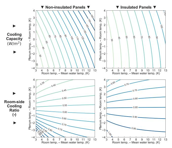
Figure 3. Developed prediction model for the tested panels.
