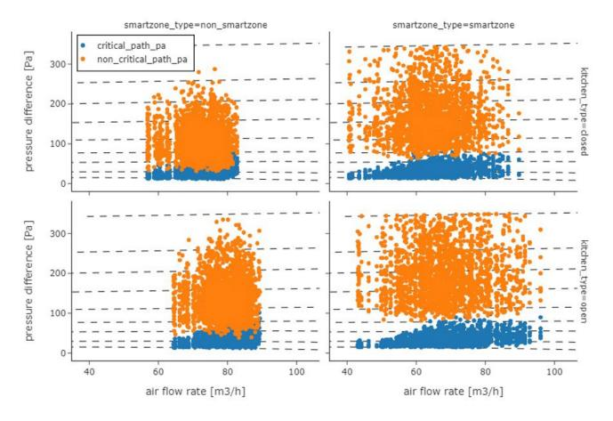
**Figure 2.** Average operating pressure (Pa) in function of the average airflow rate (m<sup>3</sup>/h) for four cases (closed/open kitchen and Smartzone/non-Smartzone). Ventilation system based on critical or non-critical path control. Dashed lines represent the ventilator curves at different voltages.
