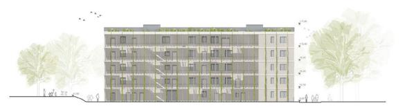
Figure 2. South elevation (top): tilted facade with solar thermal collectors and loggias; North elevation (bottom) with wooden arcade and green roof.
