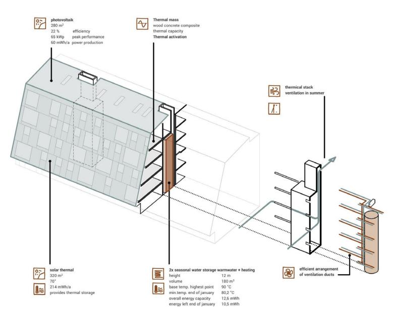
**Figure 3.** Axonometry with the different functions of the seasonal warm water storage and thermal stack – for storing heat energy and creating thermal ventilation through the storage stack in summer.
