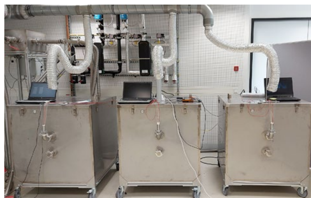
Figure 1. Emission chambers in the Air Quality Laboratory at EBC.
