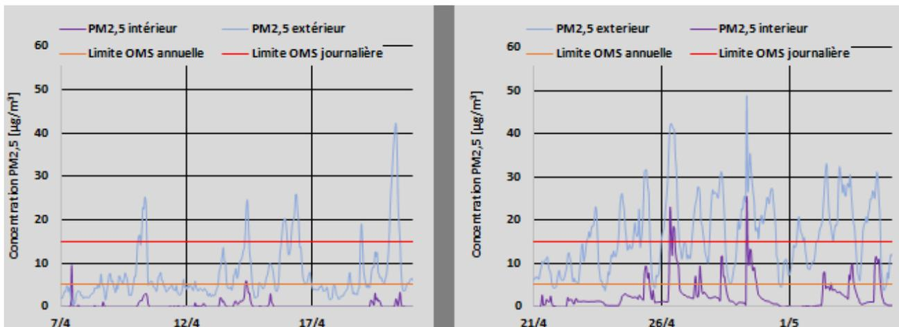
**Figure 6.** Comparative changes in the concentration of Particles Matter (PM<sub>2.5</sub>) between outdoor and indoor air, with Supply Ventilation System in operation (left) and by simply opening doors and window (right).
