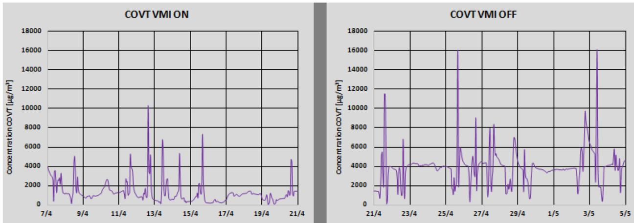
**Figure 5.** Evolution of the TVOC concentration - The curve on the left corresponds to the case where the Supply Ventilation System is in operation, the one on the right to that where the renewal of air is ensured by the opening of the doors and windows.
