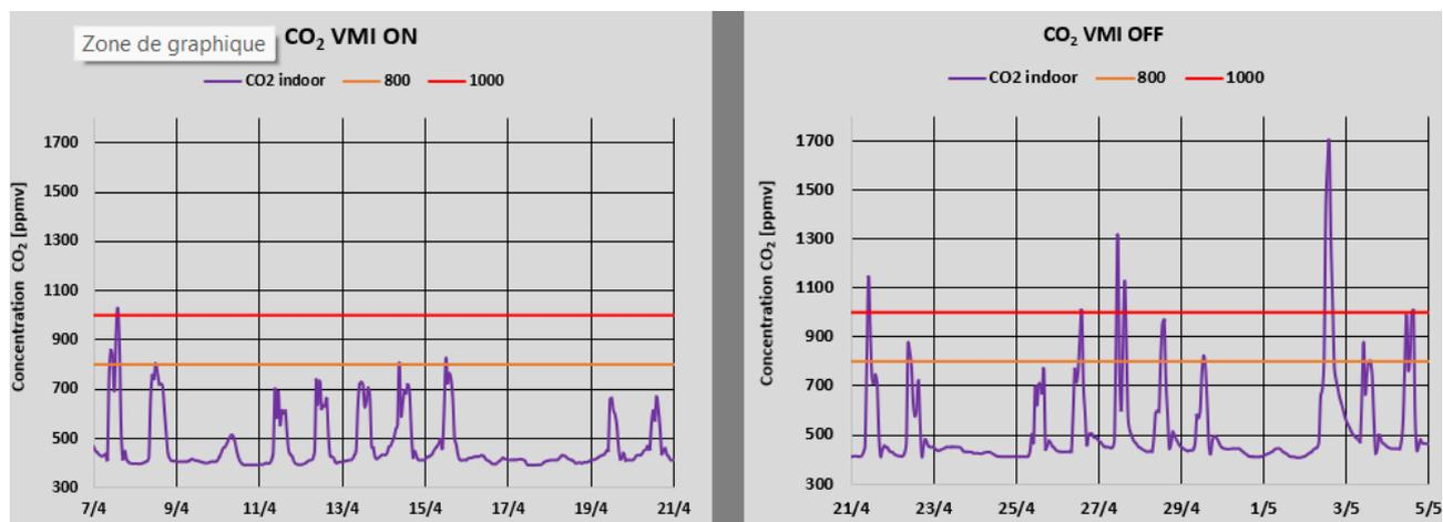
**Figure 4.** The curve on the left corresponds to the case where the Supply Ventilation System is in operation, the one on the right to that where the renewal of air is ensured by the opening of the doors and windows.
